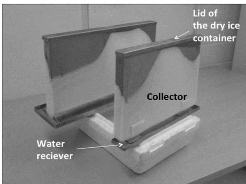
Figure 1: Two different sizes of water condensation collectors.
